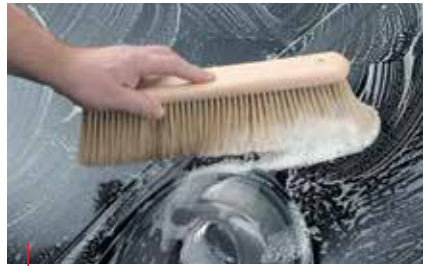
A Boar's Hair Brush is a safe and fast way to remove dirt. Boar's hair is much softer than horse hair or synthetic plastic fibers.
