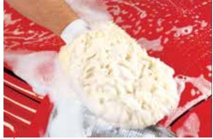
A Sheepskin Wash Mitt picks up a lot of dirt and distributes the cleaning agent evenly over the surface of the paint. Rinse your mitt often.
