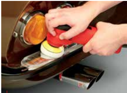
With our 3" Metal Polishing Pads and 3" Random Orbital, you can easily polish chrome and other metal in preparation for a coat of wax.
