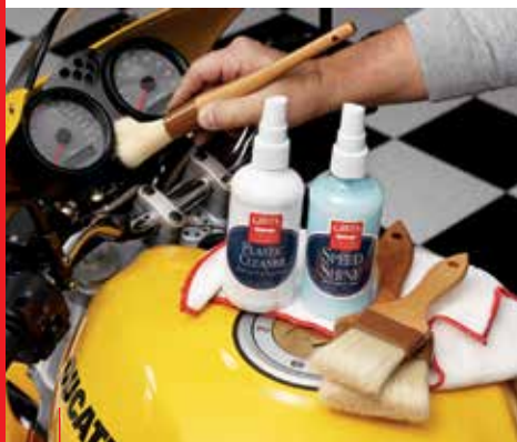
A soft boar's hair brush works well to remove light road dust from control levers and gauges.
