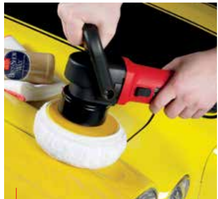
Wax Removal Bonnet fits over Blue Support Pad.
