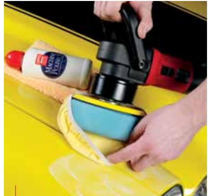
Polish Removal Bonnet fits over Blue Support Pad.
