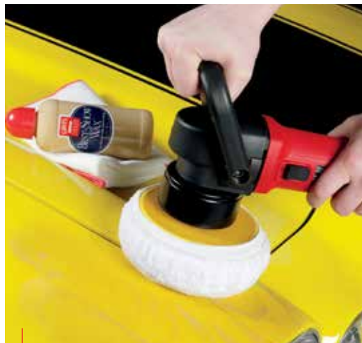
You can eliminate a lot of work by taking off the wax with our Wax Removal Bonnet and our Random Orbital. Use two or three bonnets during the process so not to allow too much wax to build up on the bonnet.
