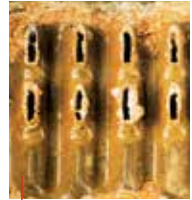
Untreated metal in your cooling system quickly builds up corrosion.
